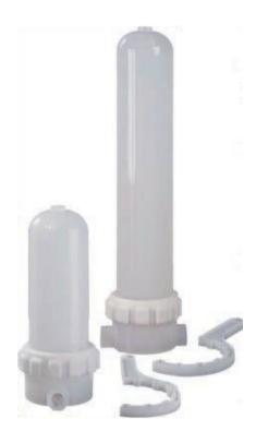
Micropore PP Filter Housing 222 type is made from pure polypropylene material, light weight and simple configuration design makes the installation and operation easier. The housing is designed to fit 10" and 20" 222 single open end cartridge. The transparent housing bowl can be easily observed with the naked eye to determine whether the internal filter cartridge need to replace. It can be used in the filtration of water and general chemicals in kinds of industry.
